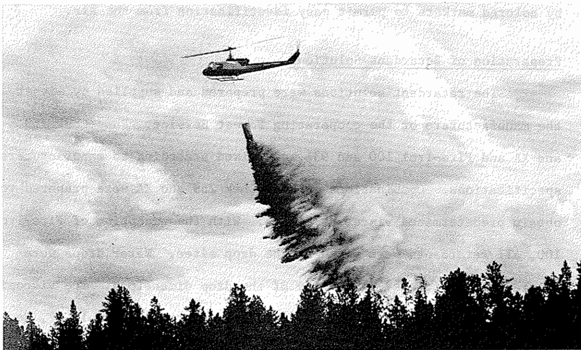
Figure 6. A drop with the Bell 204B and AFS Monsoon bucket onto a lodgepole pine stand.
