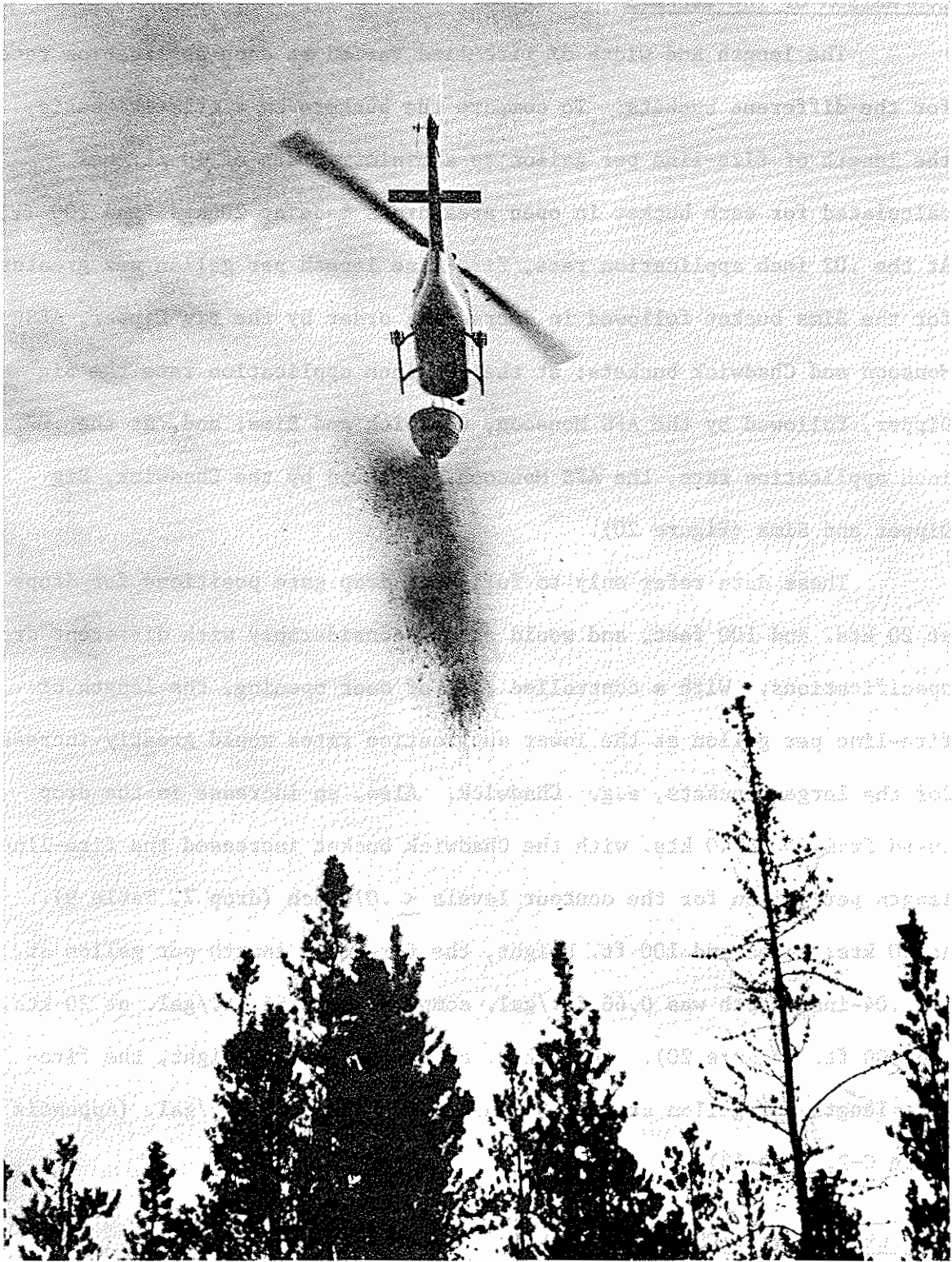
Figure 19. An air drop with the Bell 206B and Sims bucket. Note the off-centre bucket caused by correction for wind and flight path. Also note the pulsating flow of the retardant.
