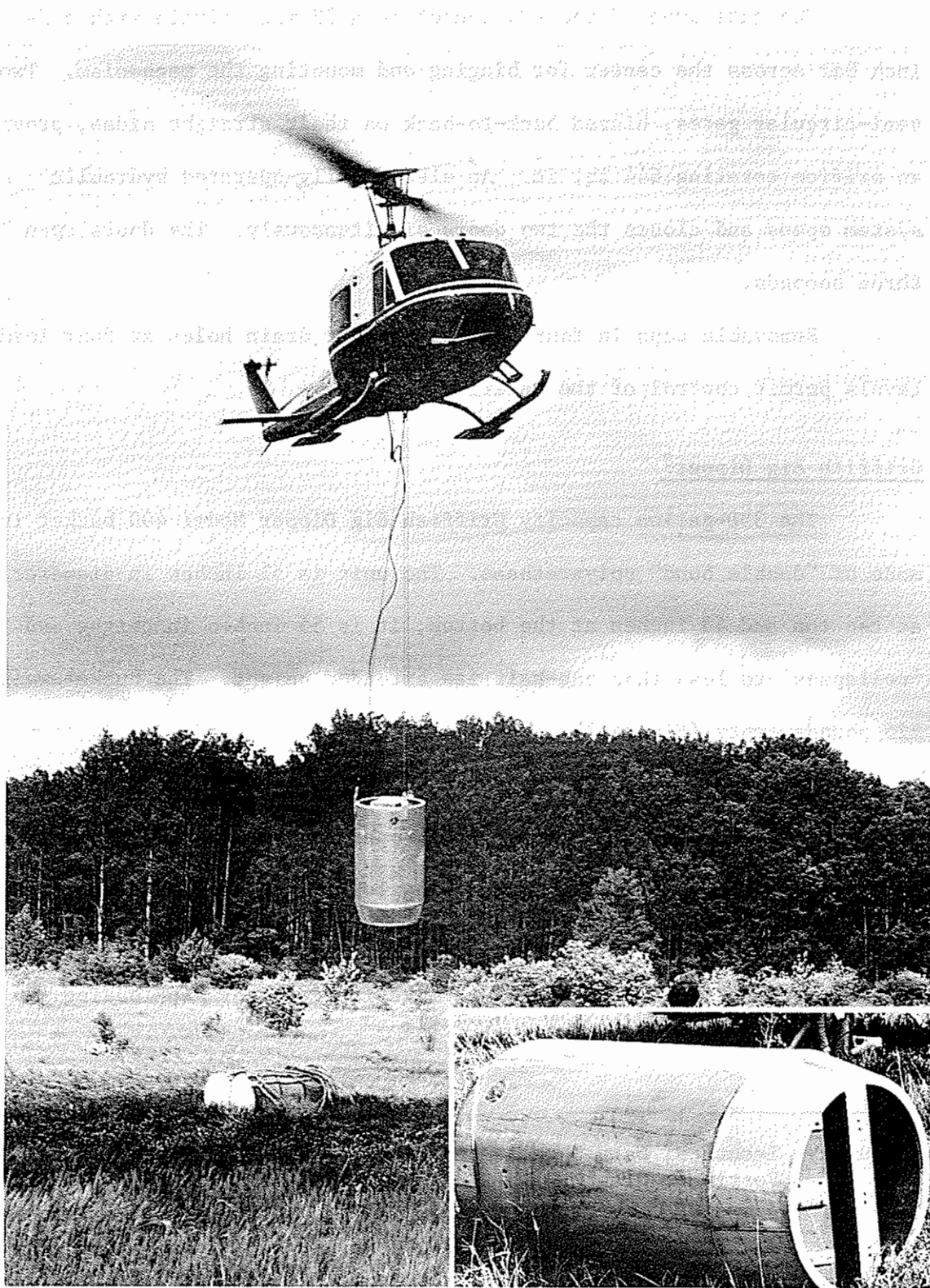
Figure 2. The 300-gallon capacity AFS Monsoon Bucket attached to a Bell 204B helicopter. Insert shows the two semi-circular doors.
